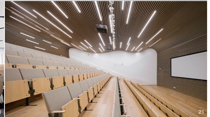
18. Trade floor view 19. Grand gallery looking down towards the grand trade floor 20. Multiple hall uses folding ceiling and incorporates lighting in proper angle to avoid direct hit on podium 21. Training room uses folding ceiling panels to reduce noise
